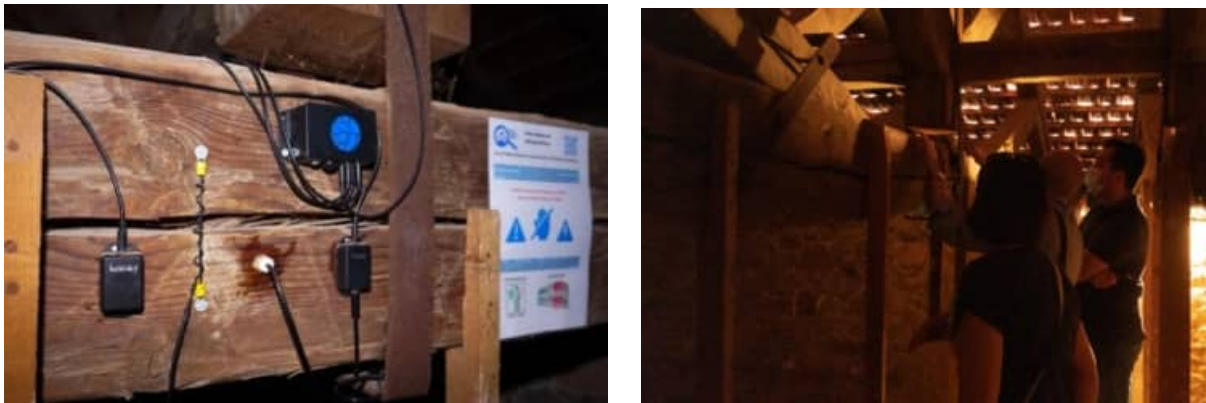
Figure 5. Installation of a “HERMON” device in a 19th-century wooden beam on a roof
