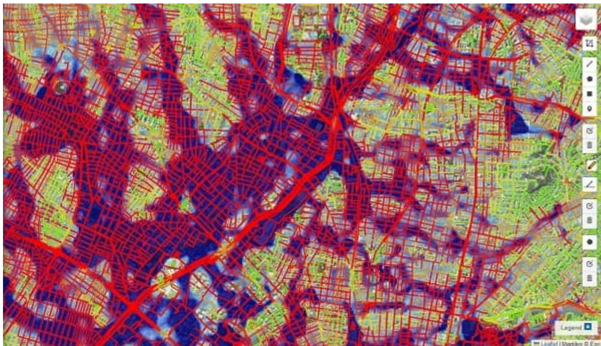
Image 11: Flooding simulation (Scenario 2 for Catchment 2 and for 1m height of full damage)
